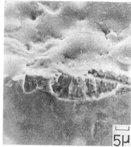
Photo. 2. SEM observation of SCC microcrack at the bottom of the artificial crevice introduced by spark machining; E=-0.2 V, K_I=4.65 MPa \cdot m ^{1/2} , after the test period of 54 ks.
